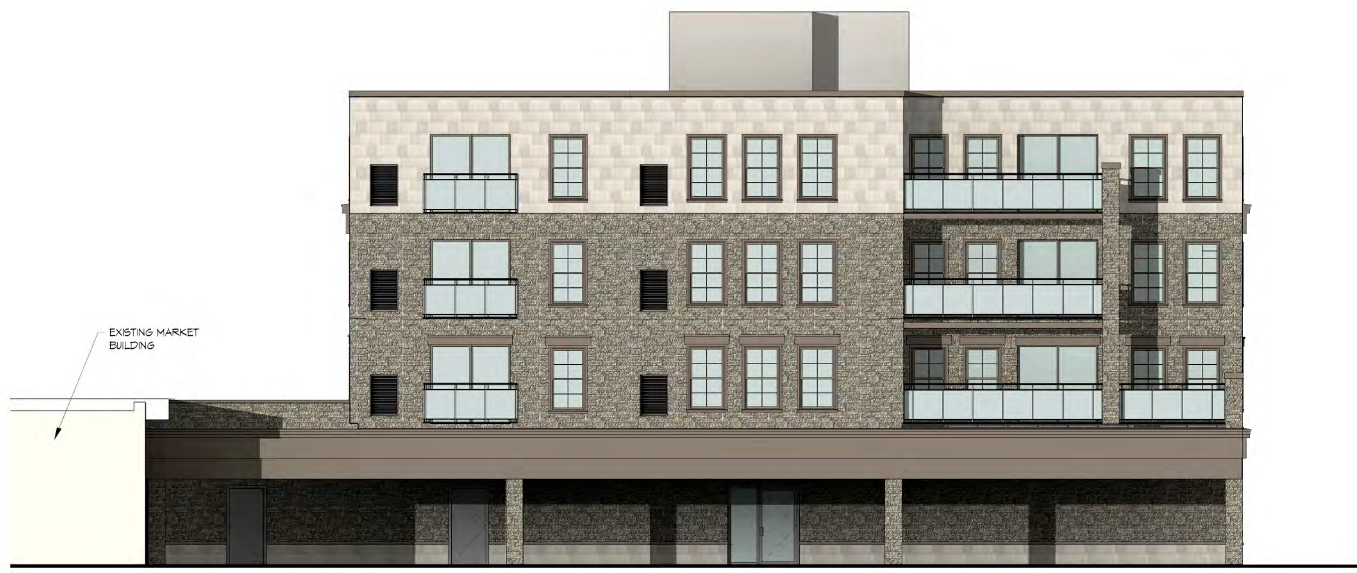
2 Geddes Bldg North Elevation SP3.0 1:100
