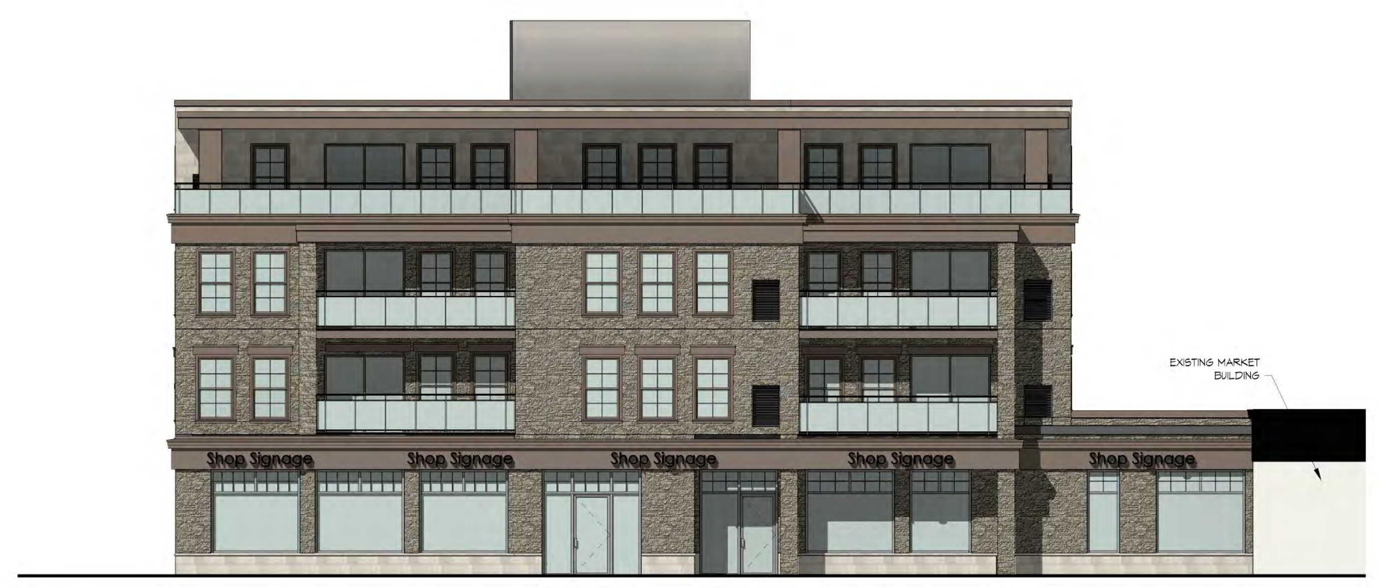
3 Geddes Bldg South Elevation SP3.0 1:100
