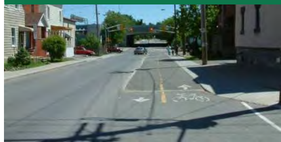
Example of a Raised Bicycle Lane on Ayres Road Source: "Cycle Tracks: Lessons Learned", Alta Planning + Design 2008
