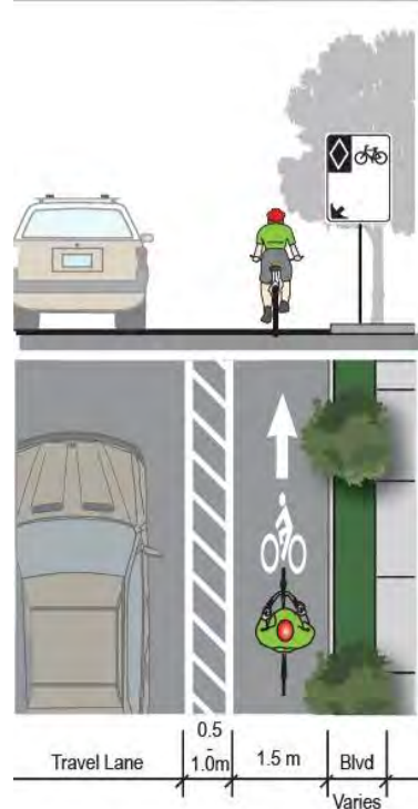
Figure 5.13 – Typical Bicycle Lane with On-Street Parking
