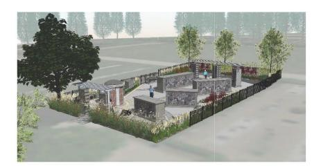
Development of the new Eden Garden cremation garden in Belsyde Cemetery will include two (2) accessible parking spaces and existing grades with slopes up to 18% improved to a maximum slope of 5% to achieve accessibility. Cemetery road width widened to facilitate vehicular travel, and improve the casket carrying distance for pallbearers.
