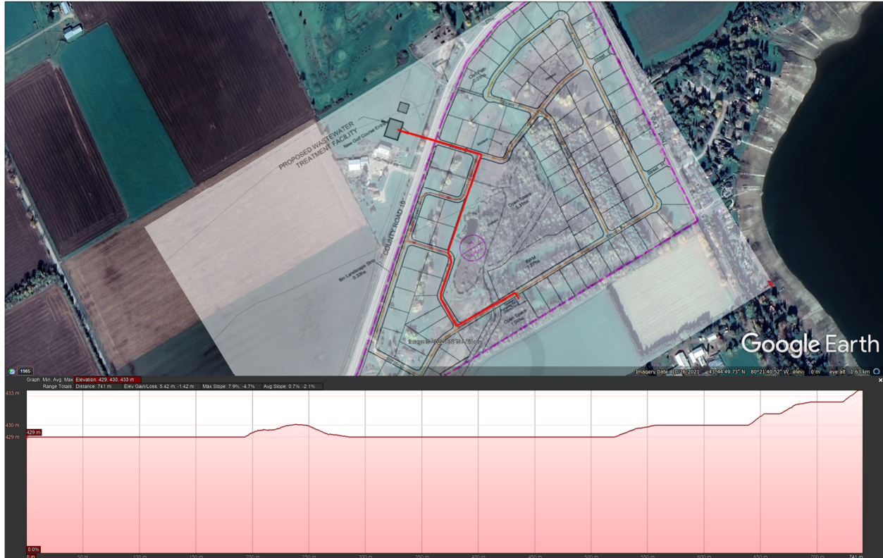
Figure 5 – Proposed Forcemain Vertical Alignment (Google Earth)
