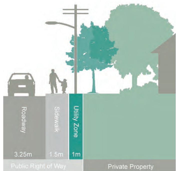
Limited Space Residential Cross Section - Within confined right-of-ways, the sidewalk is located next to the roadway and street trees are located behind the sidewalk and homeowners are encouraged to plant 'street trees' on private property.
